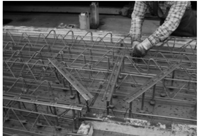
Production of precast elements using HALFEN HDB-F Shear rails
